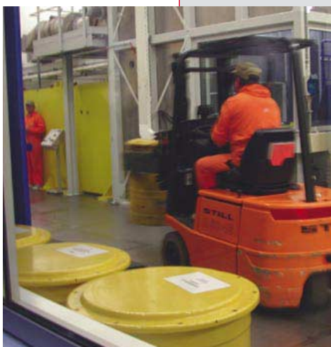
Negatively pressurized compaction room, where dismantled pieces are compacted and placed in specialized containers
